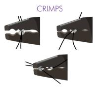
Position crimp and wire in pliers cup shaped hole. This is usually closest to handle. Squash crimp. Move squashed crimp to circle shaped hole at front of pliers, with cup facing sideways like a back to front "C" gently compress to form a ball. Test to ensure crimp is secure.
